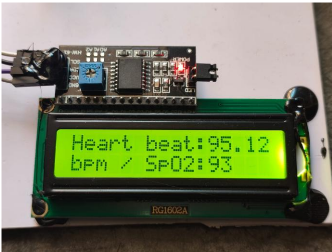
Fig - 6: LCD Display Showing Normal Heart Rate
