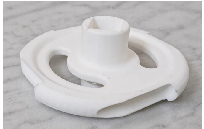
Fig – 10: 3D View of Plate Cam Designed Using Bambu Software
