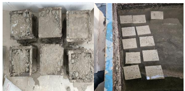
Fig-1: Casting and Curing of Specimen
